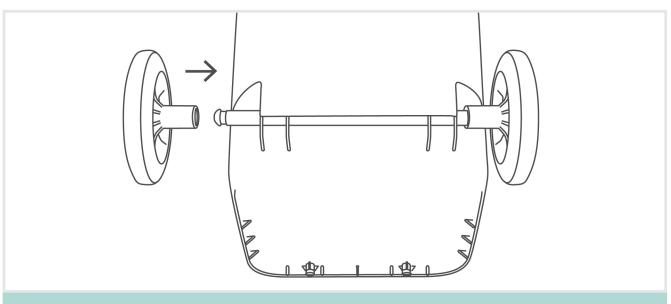
Attach the other wheel. If on correctly, the wheels should not slip off either end.
