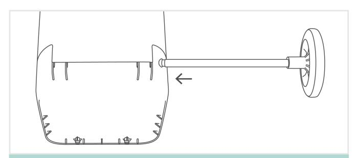
Thread the pole with one wheel attached through the holes in the bottom of the bin.
